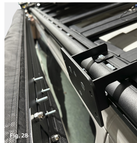
Mounting the awning on the awning bracket
