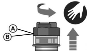
6. Unscrew the protective cap (A) (OPSO) or (OPSO / UPSO) (B) by hand.
