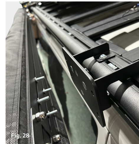
Mounting the awning on the awning bracket
