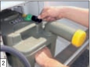
Attach the black plug to the hose connector (green). Pull out the cassette and dispose of it appropriately.
