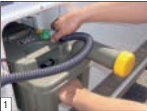
Before removing the cassette, the hose must be pulled forwards off the green hose connector.
