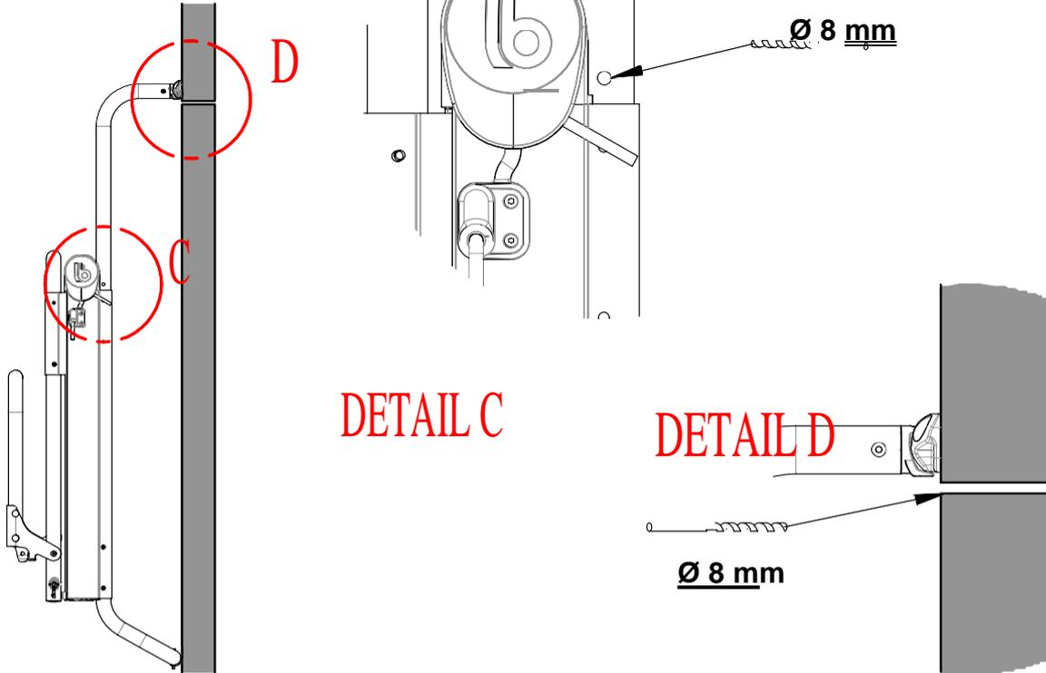
**5. remove Bike Lift from RV - insert cable in RH-arm**
