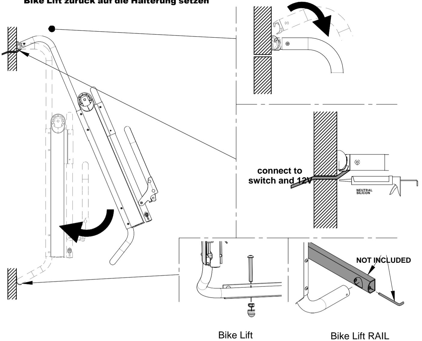
**7. wiring the motor in garage**
